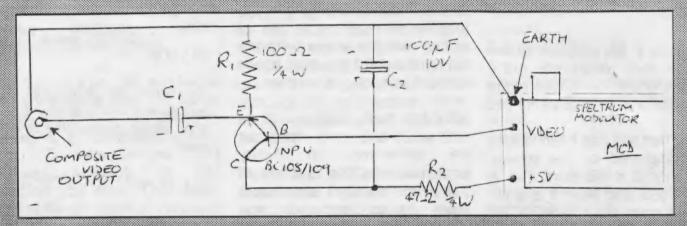
Note: Component values not critical, i.e. R1 47ohm to 200ohm R2 47ohm to 1000ohm C1 200 F to 470 F C2 100 F and up
